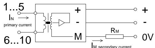
1. Output I<sub>M</sub> is positive, when the primary current I<sub>N</sub> flows in the direction from pin 1 to pin 6.
